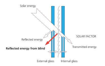
A double glazing unit with an integrated ScreenLine® blind is an excellent screen against solar radiation and offers the possibility to quickly and easily adjust the internal environmental lighting level. Due to the glass transparency, the use of normal double glazing units is often not enough to guarantee correct control of solar
